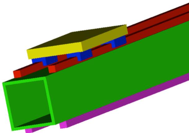
**Figure 1.** Balanced design where steel bars of same size as bearing rails are bolted on opposite side of aluminium frame member.
