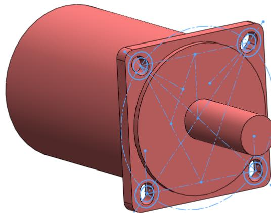
**Figure 3.** Proposed motor flange "standard" to use four slots instead of holes for split groove kinematic mounting to achieve axis alignment.
