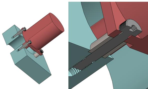
**Figure 2.** Split groove kinematic slot coupling with insulating standoffs for servo motor mounting.
