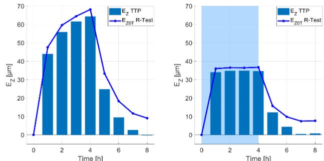
Figure 6.  $E_Z$  thermal error of the TTP as well as the MT errors measured directly after the TTP production step.
