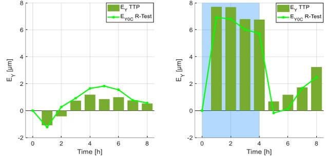
Figure 5.  $E_Y$  thermal error of the TTP as well as the MT errors measured directly after the TTP production step.
