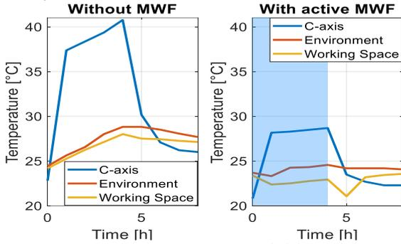
Figure 3. Temperature measurements sampled during the R-Test of both TTP experiments.
