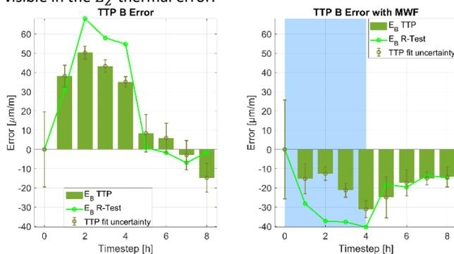
Figure 7.  $E_B$  thermal error of the TTP as well as the MT errors measured directly after the TTP production step.
