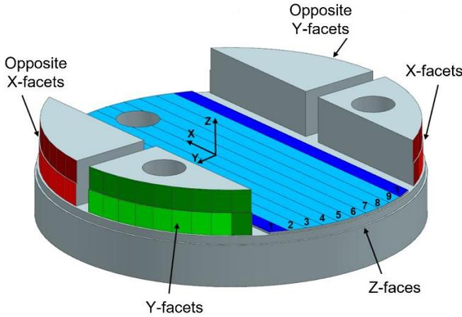
**Figure 1.** TTP with highlighted features in colours according to the respective thermal errors (red, green, blue  $\leftrightarrow$  XYZ). The darker shades depict the reference features, the lighter colours depict the eight repetitions.
