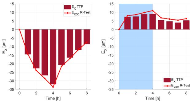
Figure 4.  $E_X$  thermal error of the TTP as well as the MT errors measured directly after the TTP production step.
