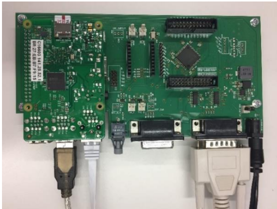
Figure 6: Raspberry Pi controller and switchbox interface.
