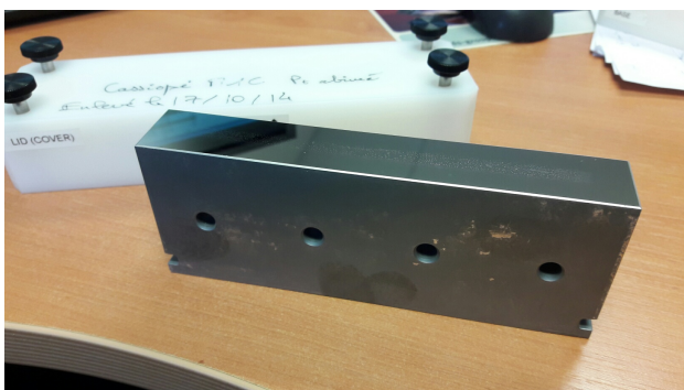
Figure 1. primary mirror for high-energy X-ray beamline (SOLEIL Synchrotron)
