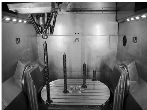
Figure 1: Measuring apparatus mounted on the tested five-axis machine tool.
