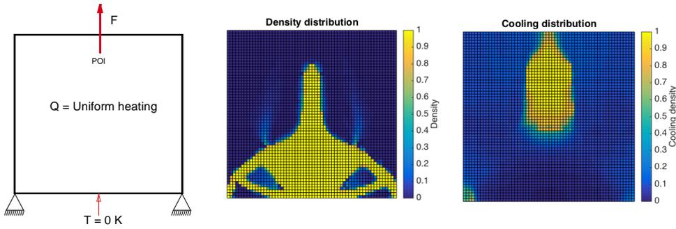
Figure 1: (left): The design domain subjected to a uniform heat load and a vertical force. The domain is fixed at the bottom corners and a heat sink is positioned in the middle of the bottom edge. The other figures present the normalized material density distribution (center) and cooling distribution (right) provided by the optimization routine to minimize the thermal error of the point of interest (POI).
