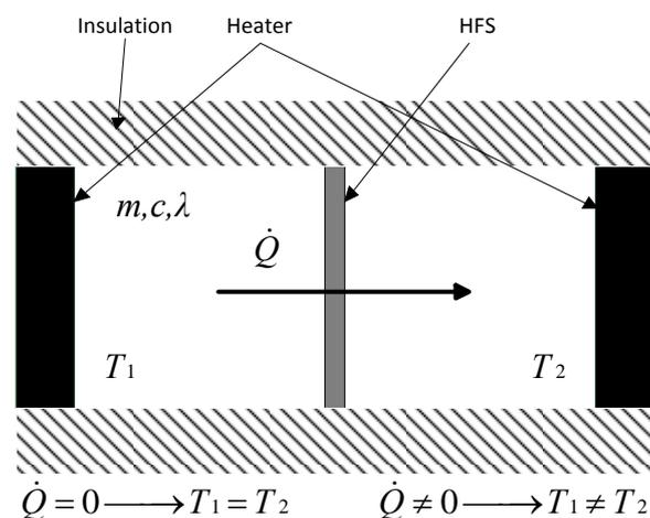
**Figure 1: Scheme of HFS with two heaters and two bodies with temperatures  $T_1$  and  $T_2$  and heat flux  $\dot{Q}$  between them.**
