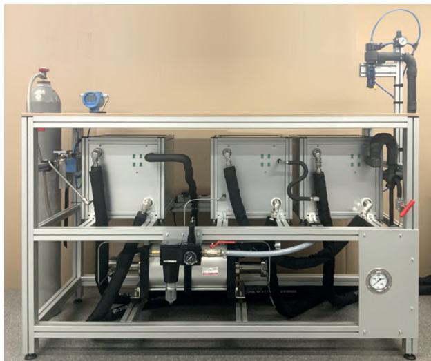
Figure 6. Newest CO 2 jet cutting equipment in Berlin developed in 2024
