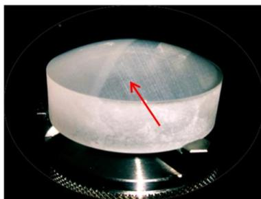
Figure 1: Half side plasma-polished aspheric lens.
