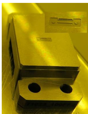
Figure 1: Mold insert with blow-up of the free-form cavity.
