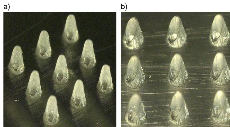
Figure 1: Two microscopic images of an injection moulded hollow polymer microneedle array in (a) front view and (b) side view.
