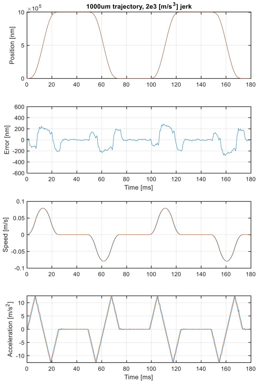
Figure 1: High dynamical trajectory tracking for one axis, 1 mm displacement within less than 30ms with a maximal tracking error of 300nm
