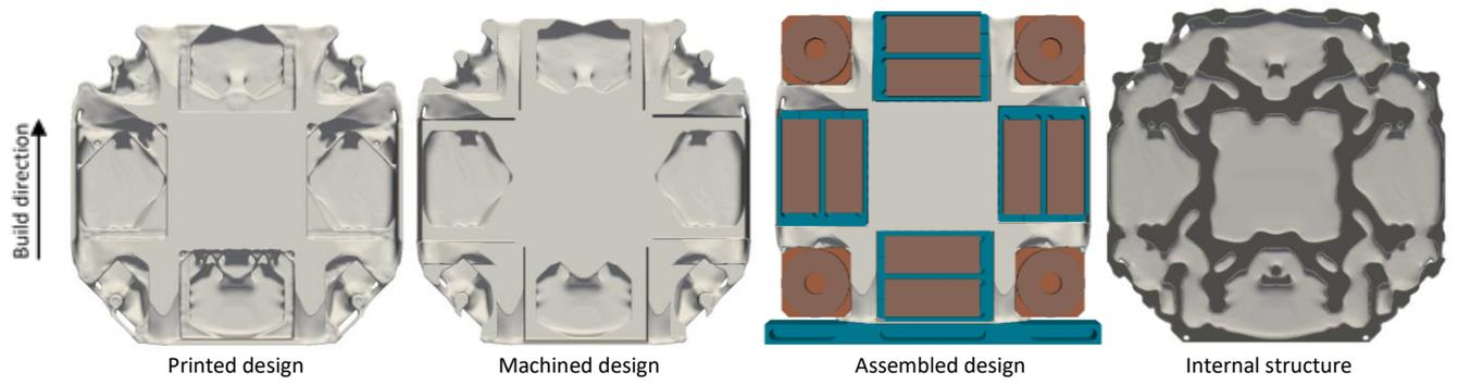
Figure 1: Overview of the final design, for different manufacturing steps of the stage
