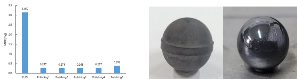
Figure 1: Comparison of material removal rate and developed ceramic ball bearing
