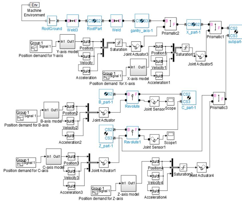
Figure 3. SIMULINK implementation of the multibody mechatronic model.
