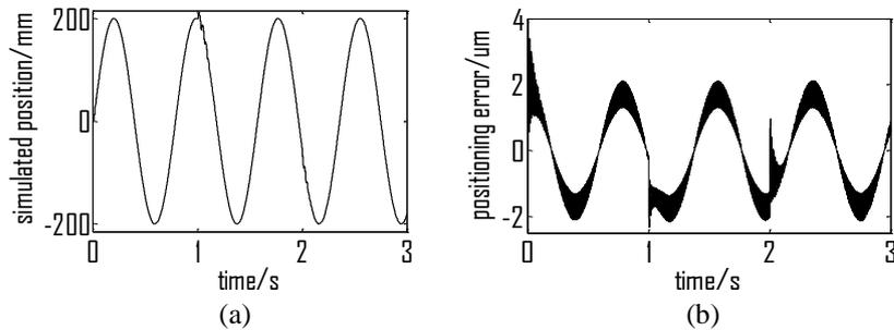
Figure 6. Simulated results for Z-axis feed drive (variable load torque); a) simulated position and b) positioning error.
