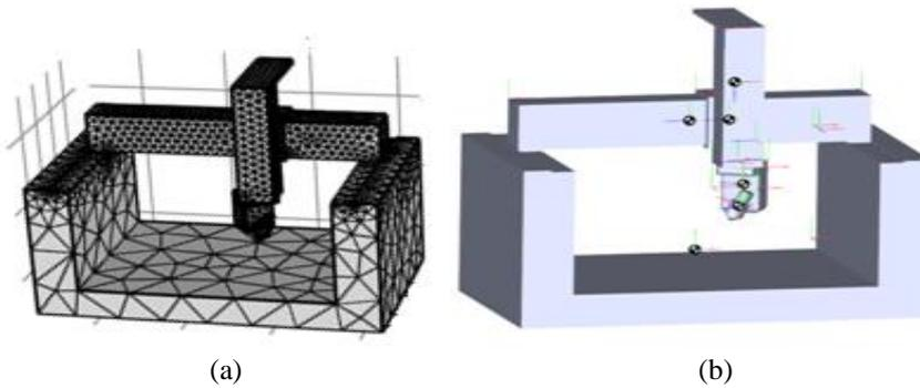
Figure 2. SolidWorks model (a) SimMechanics model (b).
