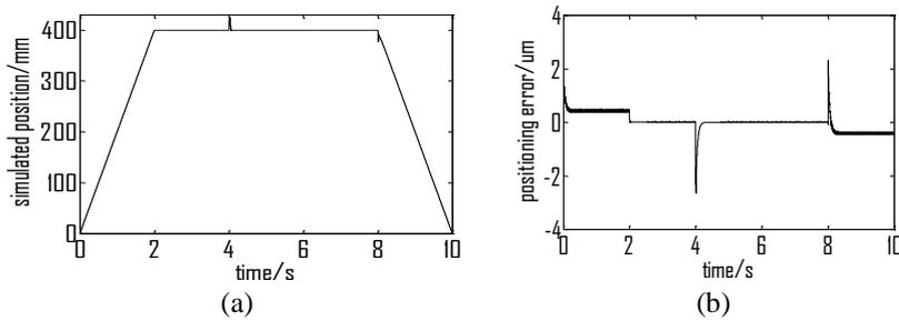
Figure 8. Simulated results for X-axis feed drive (variable load torque); a) simulated position and b) positioning error.
