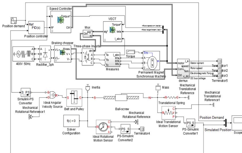
Figure 4. Details for the block 'X-axis model'.
