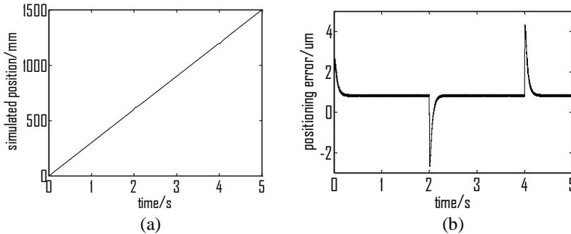
Figure 10. Simulated results for  $Y$ -axis feed drive (variable load torque); a) simulated position and b) positioning error.
