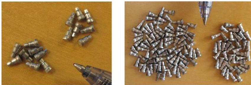
(a) Not completely formed (b) completely formed
