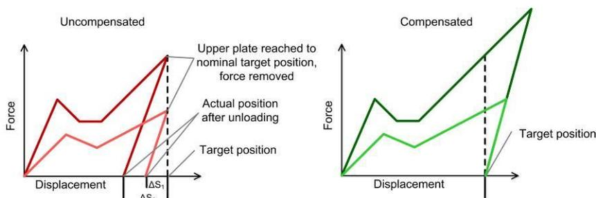
Figure 1: Concept of uncompensated and compensated elastic deflection error
