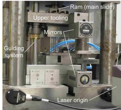
Figure 4: Experimental setup for displacement measurements under loaded and unloaded conditions
