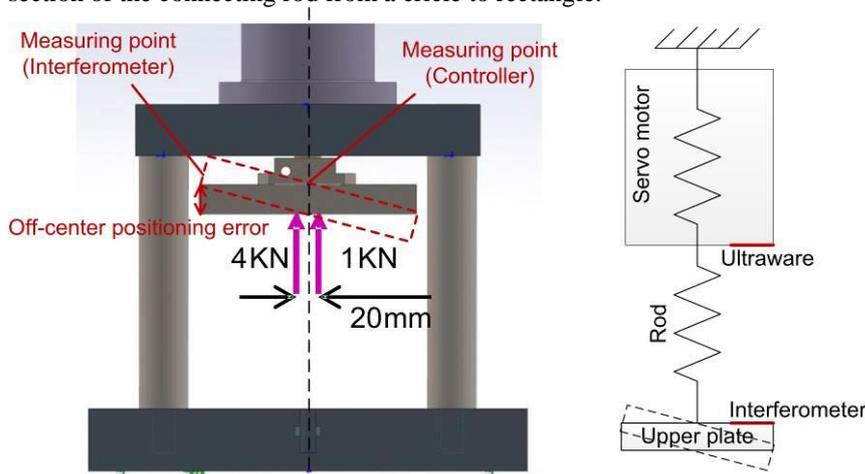
Figure 8: Measuring points on upper plate and linear servo motor for displacement
