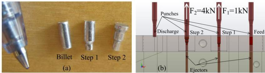
Figure 2: Forming stages; (a) Samples for billet, first and second forming stages; (b) Tooling layout and off-center loading on upper plate
