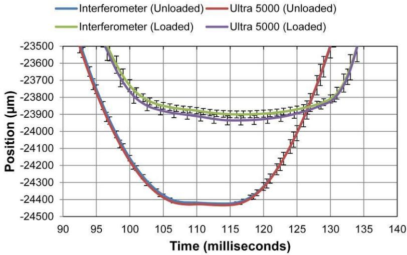
(a) Drift correction in the displacement curves
