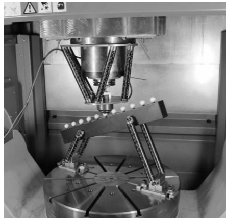
Figure 1: Spindle and artefact fixture mounted on tested machine.
