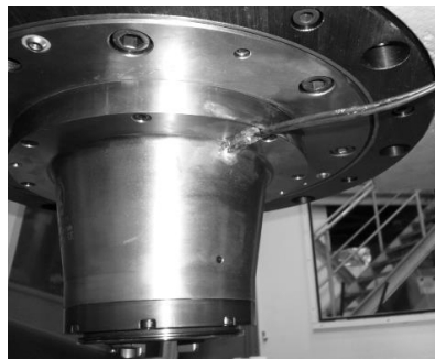
Figure 2: Placement of spindle thermal probe
