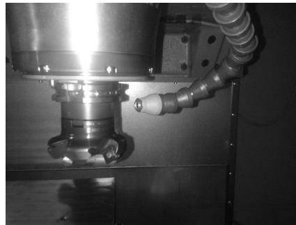
Figure 5: Used 5 edge cutter and the infrared sensor placement
