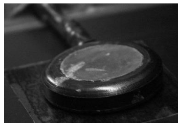
Figure 7: The detail of used heat transfer coefficient sensor
