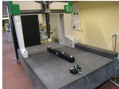
Figure 4: Setup of the sphere beam along the x axis of a CMM.
