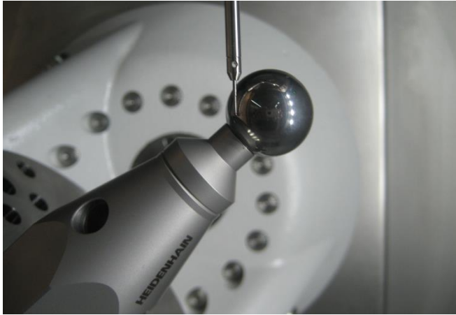
Figure 7: B-axis calibration with touch probe and calibration sphere
