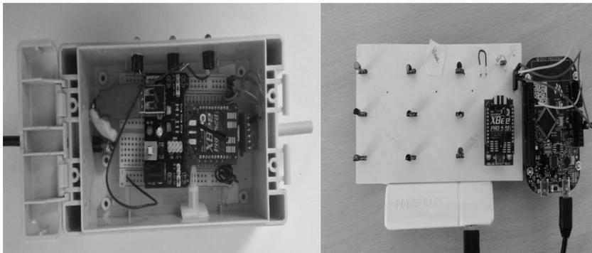
Figure 4 Left: ZigBee coordinator. Right: transmitter to system.
