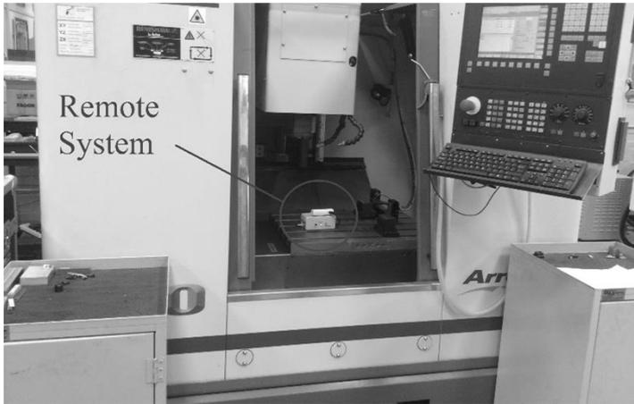
Figure 7: A Picture of the Remote System on the Work Table of one CNC machine.
