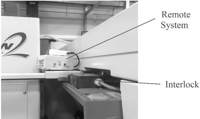
Figure 5: A Picture of the Remote System on the Interlock
