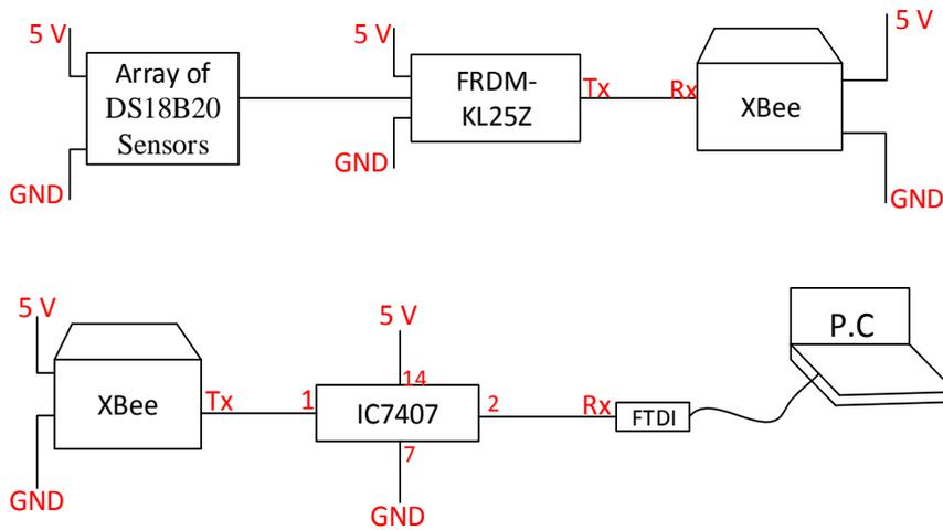
Figure 2: showing the wireless sensor setup
