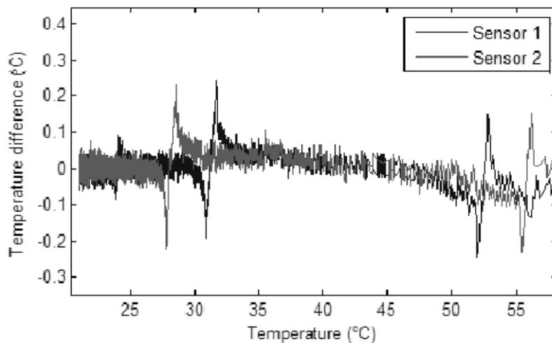
Figure 1: Error in the readings of two DS18B20 sensors when compared to a standards level thermistor (FLUKE CHUB E4 1529 controller and 4-Wire thermistor)
