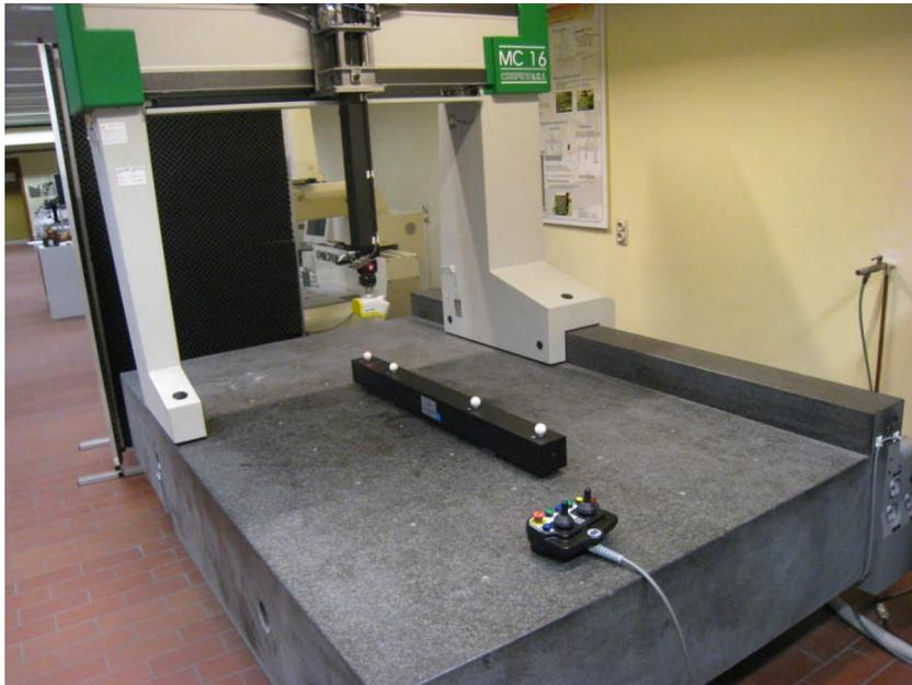
Figure 1: Setup used in the study: CMM, laser line scanner probe mounted on rotary head and KoBa sphere beam.
