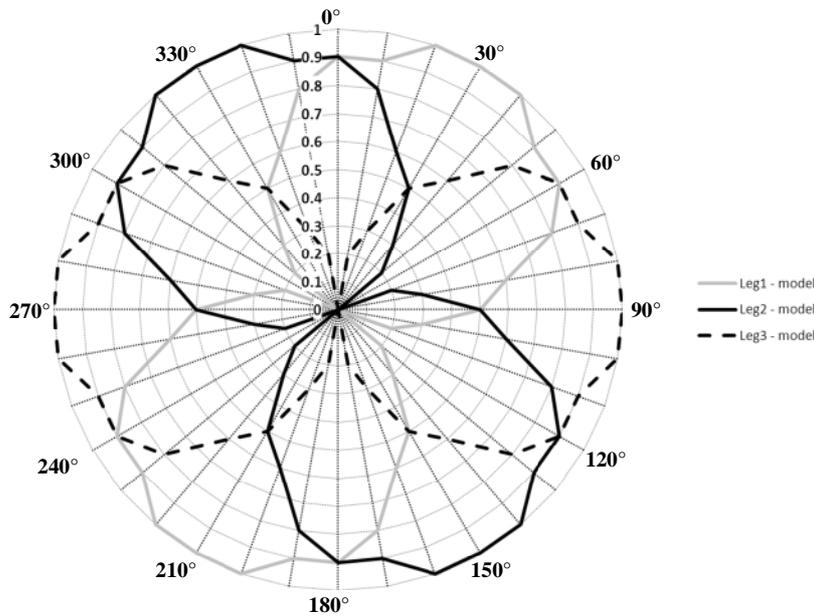
Figure 5: absolute values of vibration amplitude, as calculated by the vibration control algorithm. The radial axis indicates relative vibration amplitudes, and the azimuthal axis indicates vibration vector.
