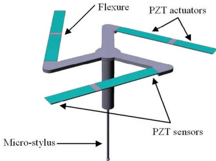
**Figure 1:** Schema of the NPL micro-CMM probe.
