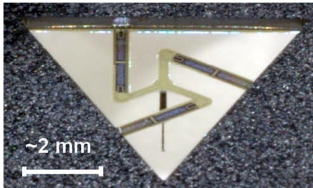
**Figure 2:** An assembled micro-CMM probe.
