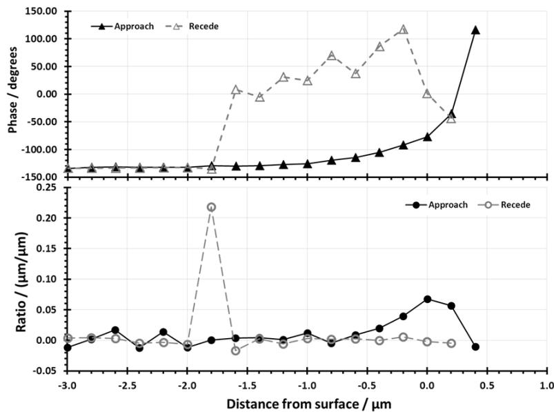
**Figure 4:** Lateral test results in one lateral vibration direction. Comparison of the two measured signals: phase of the output signal relative to the drive signal (top) and the amplitude measurement (bottom), plotted against distance from surface.
