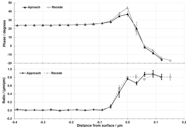
**Figure 3:** Vertical test results. Comparison of the two measured signals: phase of the output signal relative to the drive signal (top) and the amplitude measurement (bottom), plotted against distance from surface.
