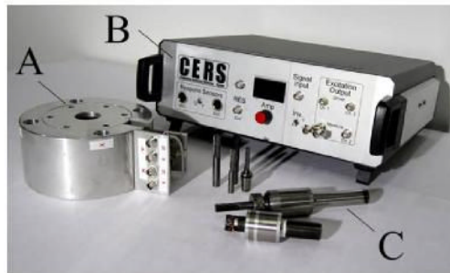
Figure 1: The contactless excitations and response system CERS: (A) actuator hardware with on-board displacement sensors; (B) actuator and sensor control system; and (C) specially developed cutting tools.
