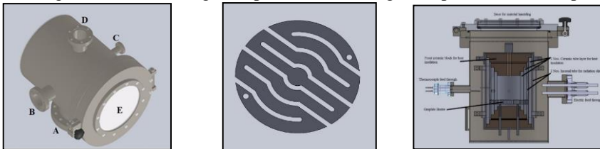
Figure 1. CAD of a) chamber, b) graphite heater, c) furnace assembly
