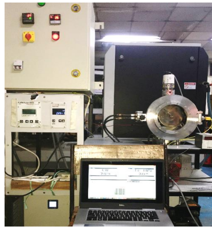
Figure 4. Assembly of vacuum brazing furnace
