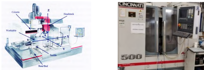
Figure 1 : Machine Tool Configuration (Left) and Cincinnati Arrow 500 (Right) [8]
