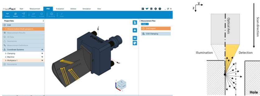
Figure 1: Left: Turbine blade with different kinds of holes. Yellow arrows show typical measurement directions which are parallel to the hole axis using VFP. Right: VFP measurement principle.
