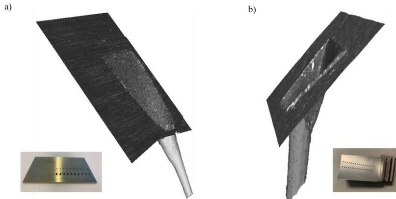
Figure 3: 3D measurements of cooling holes by FV and VFP. The FV measurement of the top surface is fused with the VFP measurement of the hole. a) Cooling hole of the measurement artefact. b) Cooling hole of a turbine blade.
