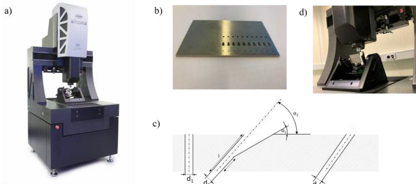
Figure 2: a) Bruker Alicona  $\mu\text{CMM}$ . b) Measurement artefact. c) Schematic cross section of the plate. d) Experimental setup.
