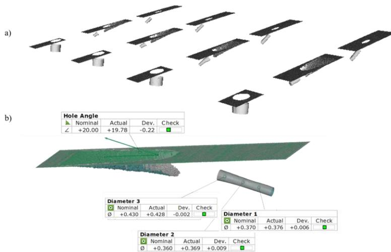
Figure 4: a) Multi-measurement on the plate. b) Geometric verification exemplarily for a fan-shaped cooling hole.
