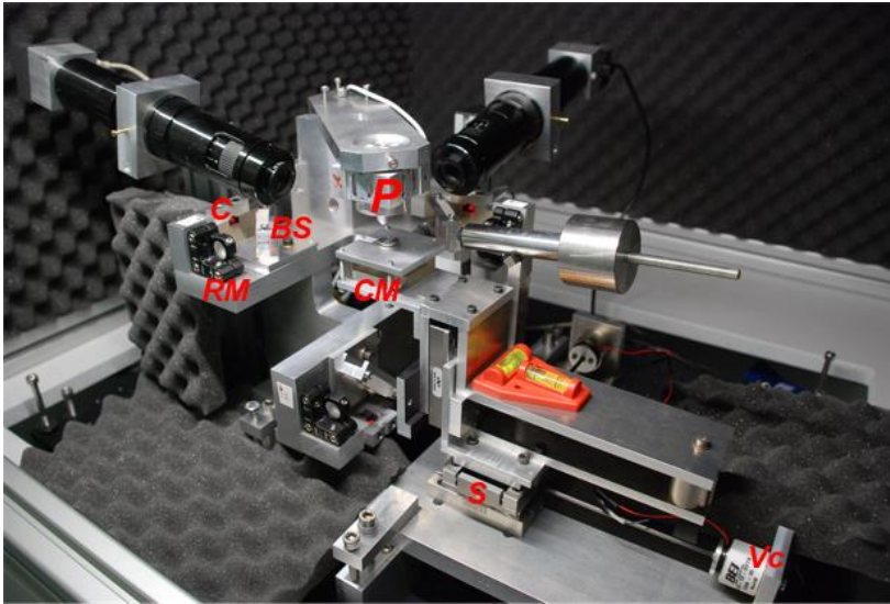
Figure 9. The realized \mu CMM system ( P : Probe; CM : Corner mirror; C : Camera; BS : Beam splitter; RM : Reference mirror; Vc : Voice coil actuator; S : Newport UMR stage)
