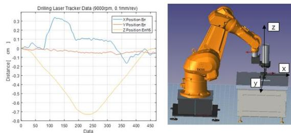
Fig. 3. Position error data of laser tracker during robot drilling.
