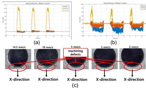
Fig. 2. (a) Machining load of the machining center, (b) Machining load of the robot manipulator, and (c) Robot drilling defects in various conditions.
