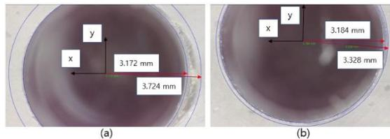
Fig. 4. Comparison of defects in the hole entrance before and after applying the algorithm
