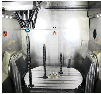
Figure 2: Volumetric error measuring of 5-axis machining centre using MT-Check probe and calibrated spheres placed across the workspace [5]
