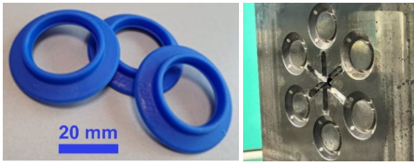
Figure 1. Precision moulded polypropylene ring (left); six-cavity two-plates cold-runner mould (left).
