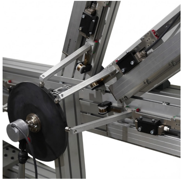
Figure 3. Reference steel disk mounted on the presented roundness measuring device. The disk was rotated with small electric motor and supported by two ball bearings. Encoder is directly attached to the steel disk.
