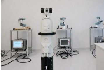
Figure 1a) Testing the robot in accordance with PN-EN ISO 9283:2003, using the Lieca LTD 840 tracking system, Figure
