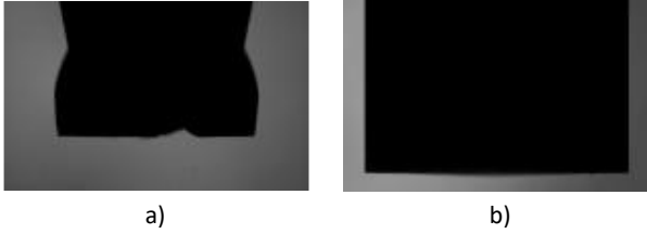
Figure 2. Silhouette images captured by the system of a) a 3 mm, four-fluted flat endmill and b) a square bar at 6000 rpm.
