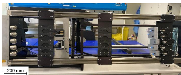
Figure 1. Overall view of the 9-axis Coater Mk2, with one balloon catheter mounted
