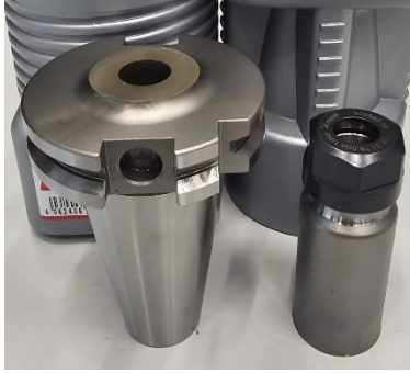
Figure 2. Axially shortened tool holder, HOLEX SK40 ER16.
