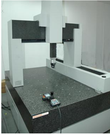
Figure 1. Five-axis coordinate system utilized during experiments consisting of Zeiss WMM 850S with installed probing system Renishaw PH20.
