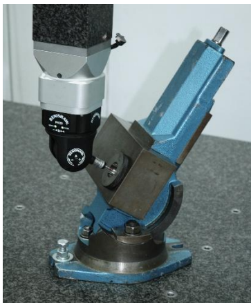
Figure 2. Five-axis coordinate system utilized during experiments consisting of Zeiss WMM 850S with installed probing system Renishaw PH20.
