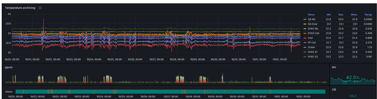
Figure 2. Environment sensor monitoring and history panel. Two weeks of data are shown. Top: temperature sensors; middle: particle counts and relative humidity; bottom: lab door status and control room temperature.
