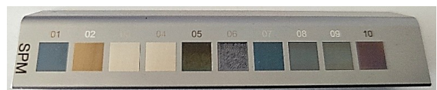
Figure 4: Test fields for ablation characterisation by laser parameter variation
