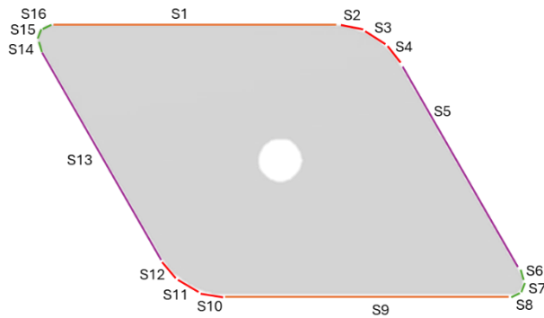
Figure 5: Example for division of the punch shell surface into 16 sub-segments to structure the rhombus punches
