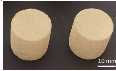
Figure 3. Printed cylindrical specimen ( \varnothing 20 mm \times 20 mm) from the optimised 60 wt% fine fraction blend.
