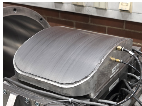
Figure 1. A bearing finished with abrasive film installed in the measurement setup.
