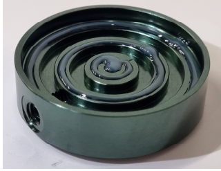
Figure 1. Anodised aluminium bearing body with air supply grooves. Epoxy adhesive applied with a robot [11].
