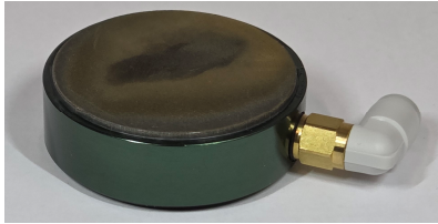
Figure 2. Porous metal restrictor cut with wire EDM joined to the bearing body with adhesive.
