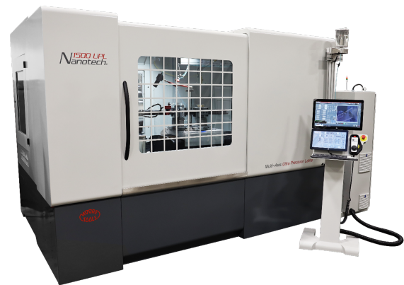
Figure 5. 1500 UPL, the largest ultra precision machine [5]
