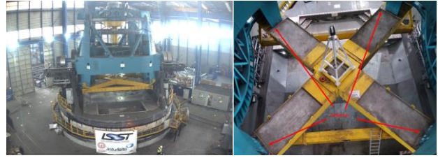
Figure 8. TMA real survey scenario (left) and laser tracker placed within the TMA and a detailed view of the laser tracker positioned within the TMA alongside reflectors mounted on the M1M3 dummy (right).
