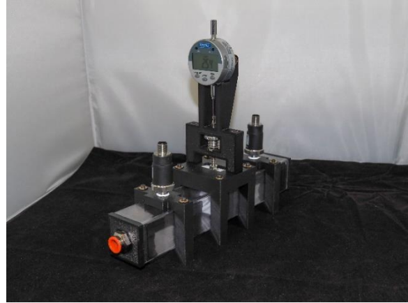
Figure 6. Flow characterization test assembly
