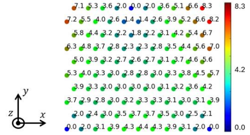
Figure 2. Uncertainty Propagation Factors for each node of a 10x10 grid considering equal uncertainty for all measurements. The nodes are represented in the corresponding xy position.
