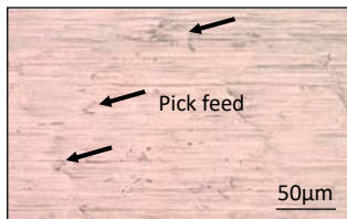
Figure 14. Machined surface obtained with flow velocity of 95 m/s at cutting distance of 990 m
