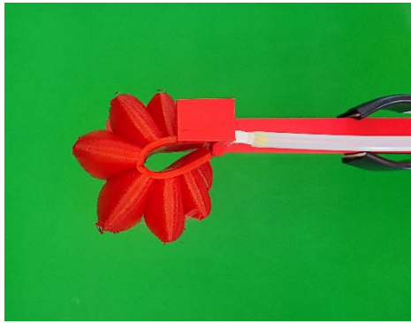
Figure 8 The soft actuator under 0.1578 MPa pressure
