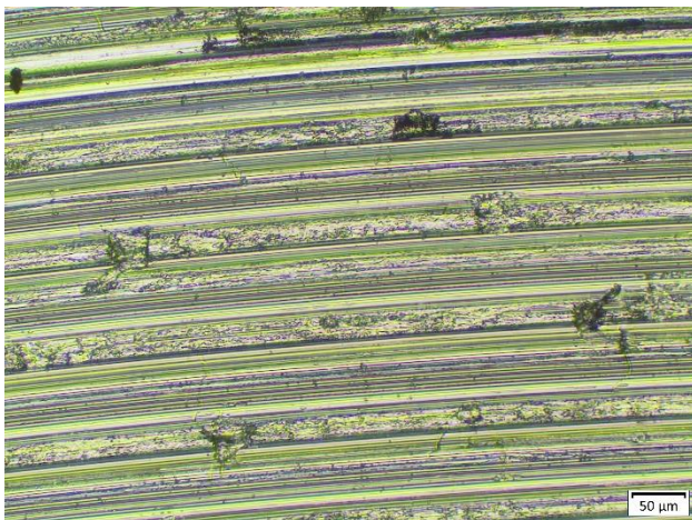
Figure 4. Turned surface of sample 8 with 180 \mu\text{m} hatch spacing.
