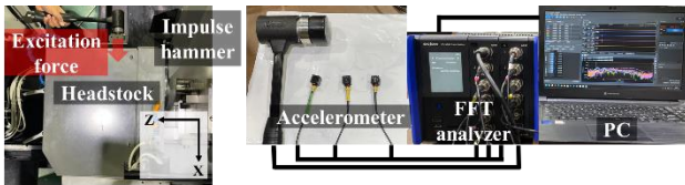
Figure 3. Experimental modal analysis setup
